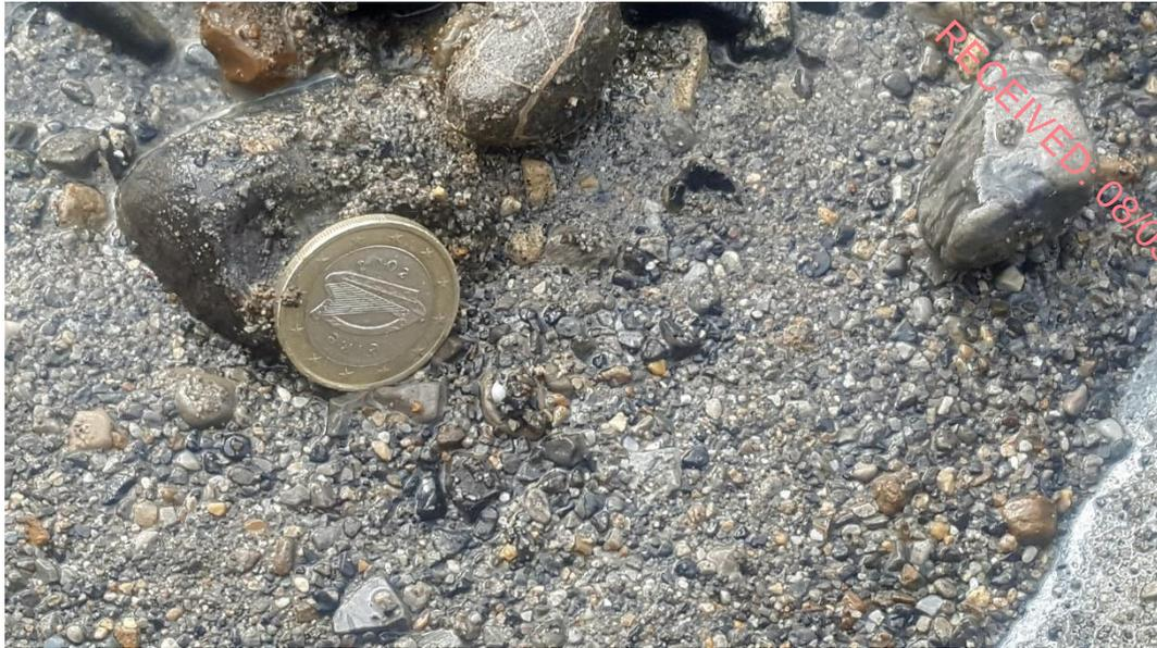
Figure 13. Washed trial pit sample
