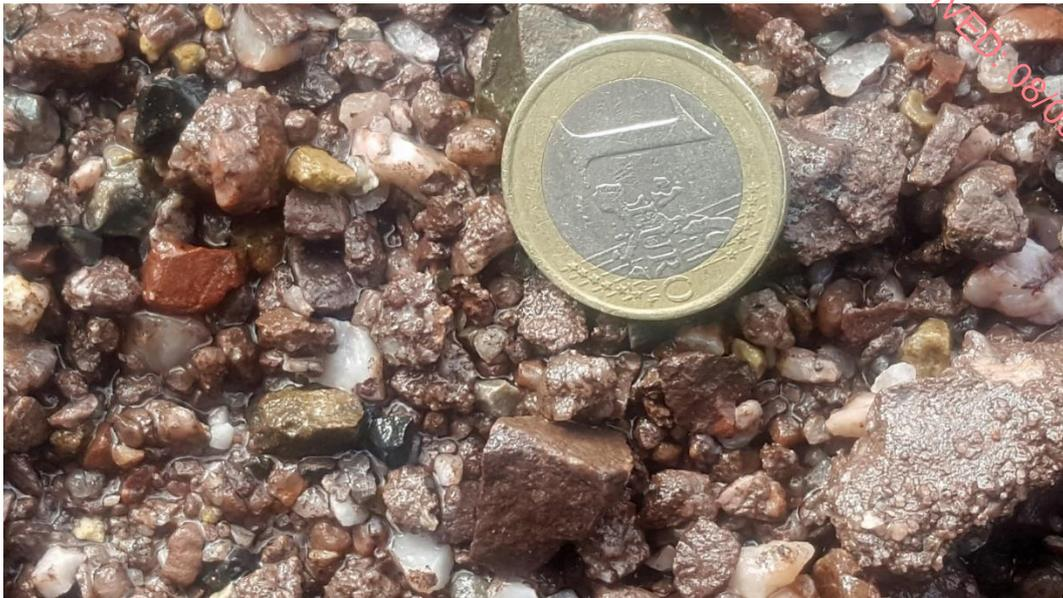
*Figure 11. Red Sandstone bedrock in BH2. There is also quite a lot of white vein quartz. A few exotic fragments including the green andesite, behind the €1 coin may have fallen down the hole.*
