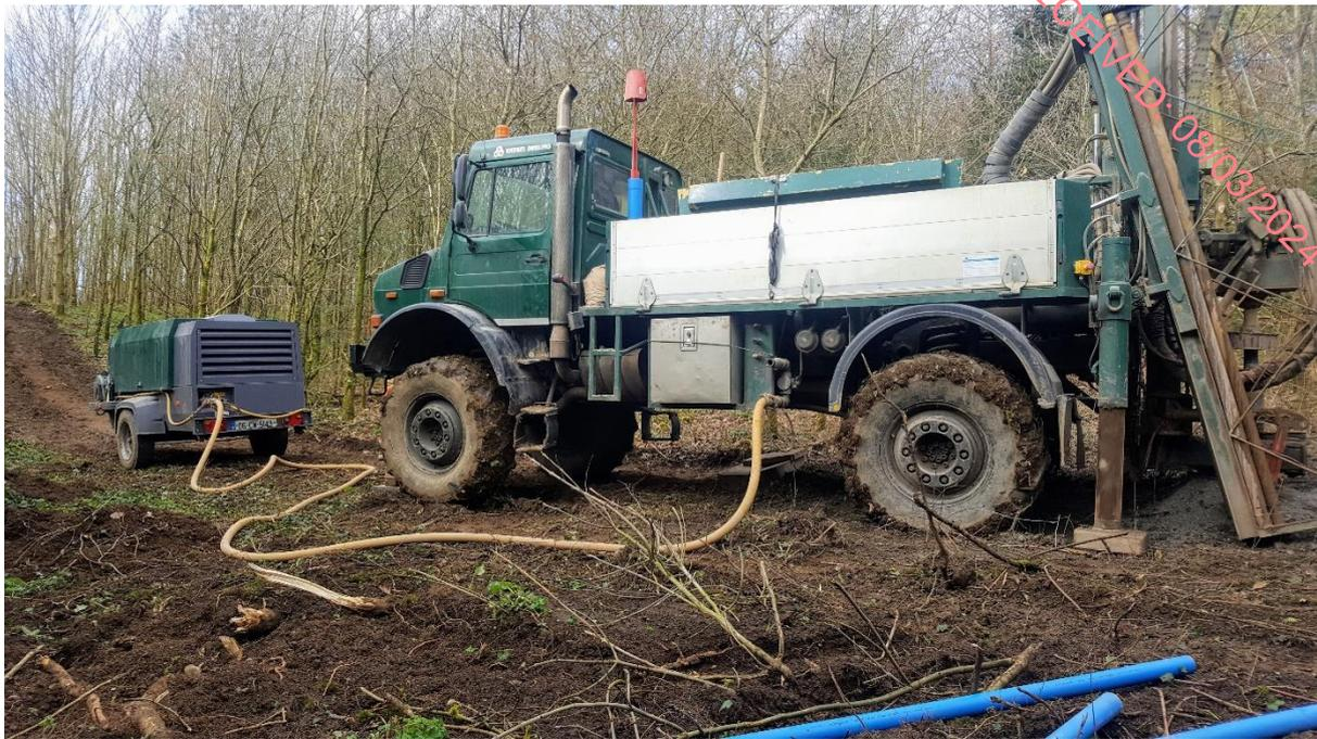
*Figure 5. Drill rig in operation on the site of BH5*
