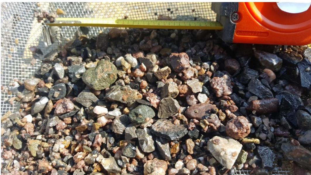
Figure 10. Washed material from 29.5m in BH2. Note pieces of red sandstone, vein quartz, and Ordovician andesite
