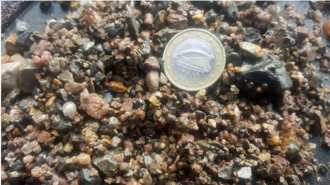
*Figure 11. Washed sand and gravel, 10m, BH5*
