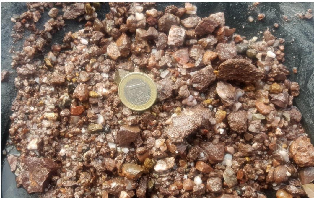
*Figure 10. Red sandstone bedrock in BH3.*
