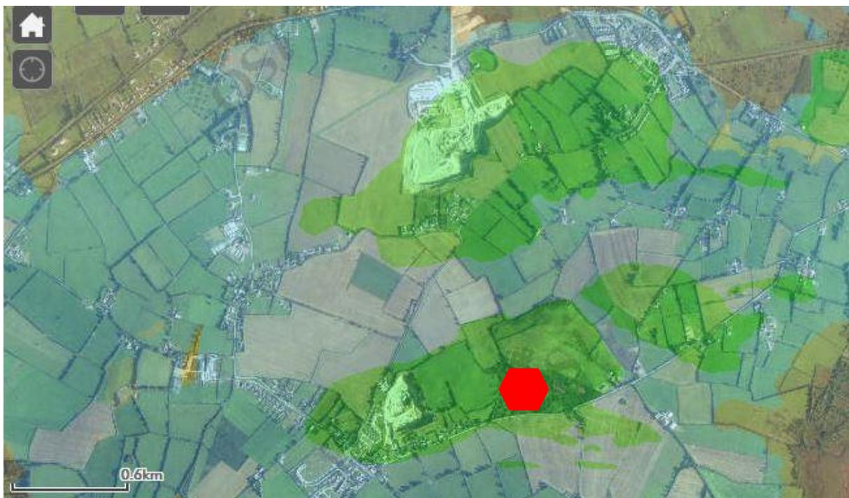
Figure 3. Quaternary Geology of the area around Kilmeague taken from the Geological Survey of Ireland. Sand and gravel deposits are in green, till in pale blue-green, and peat in brown. Note the large gravel pit (Hanlon Concrete Products) north of the site and the exhausted pit, west of the site.
