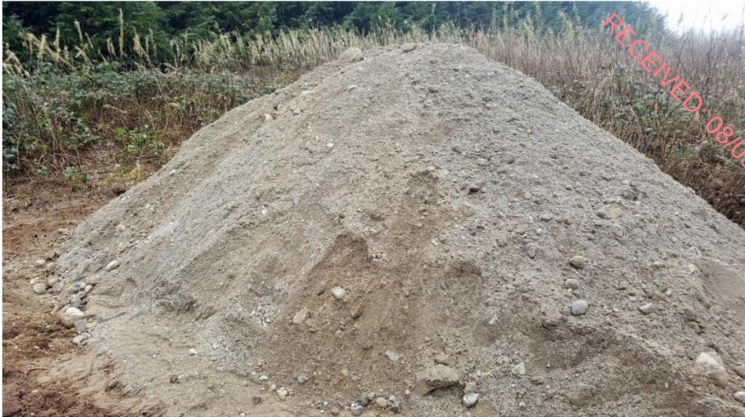
*Figure 7. Sand and gravel extracted from the trial pit.*
